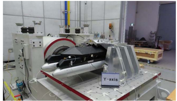
Fig. 14 Dynamic load test configuration
